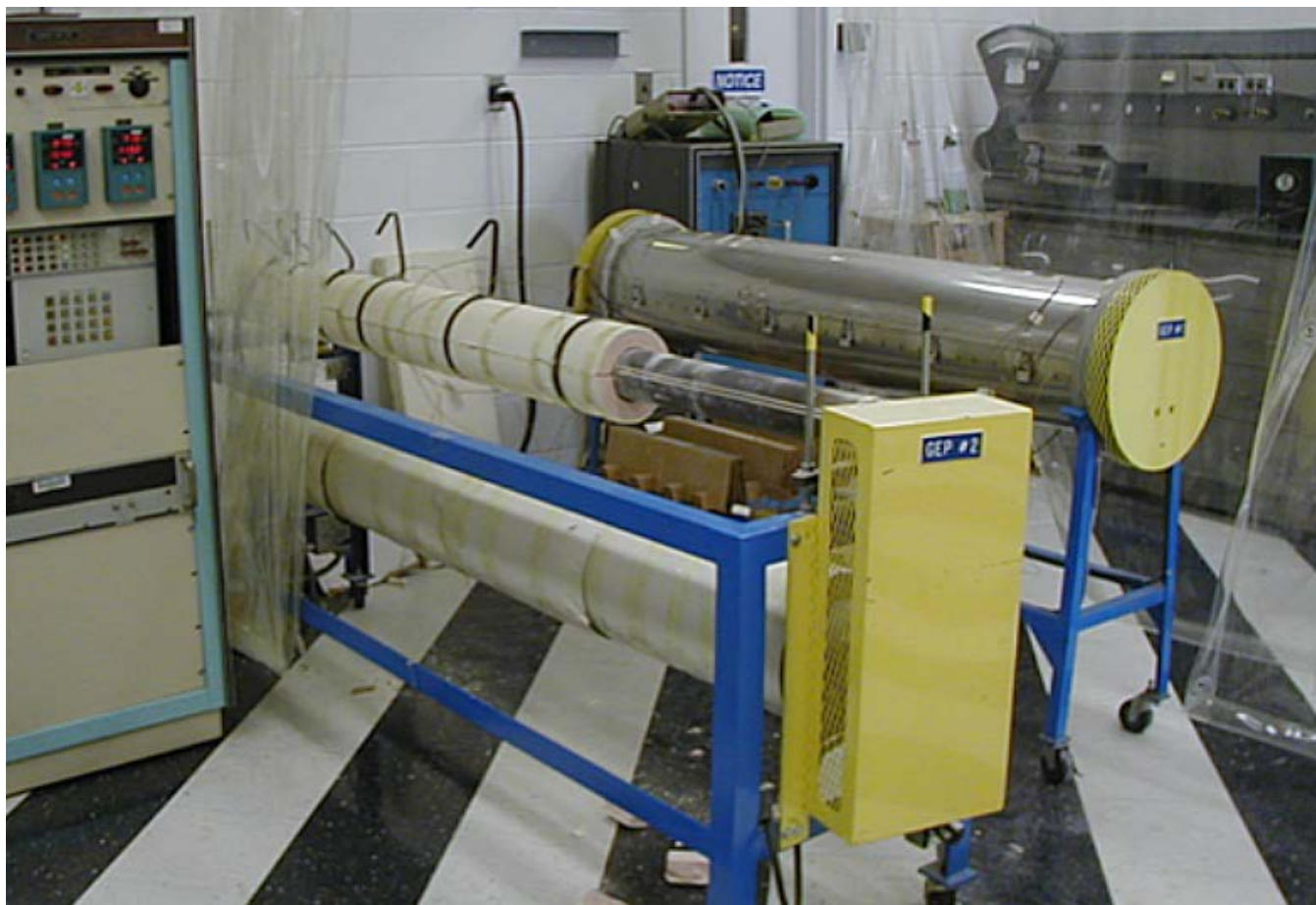
Figure 5: Guarded end apparatus used to measure the transfer of heat through the insulation for ASTM test method C335. Designed for pipe insulation.
