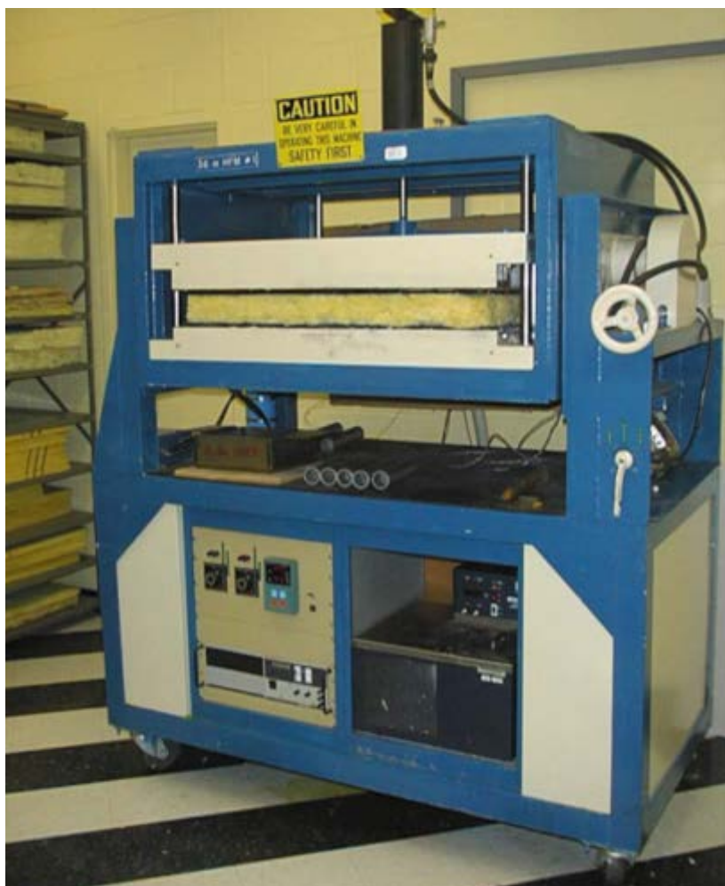
Figure 4: Heat flow meter used to measure the transfer of heat through the insulation for ASTM test method C518. Designed for boards, blankets, & blocks.
